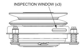
Figure 6-3. Clutch Air Gap Adjustment
